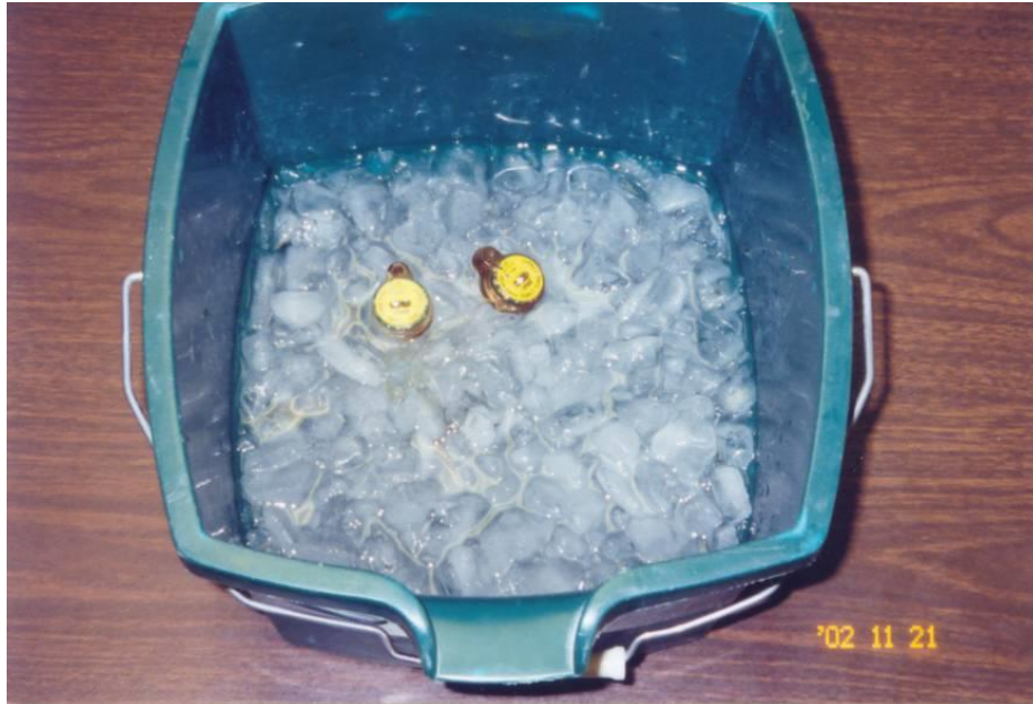
Figure 8-100. Picture of Crushed Ice Bath that was used as a QA Check to Determine if the Temperature Loggers were Performing Within Acceptable Limits. Loggers were Submerged into the Ice Bath and the Bucket was Placed in a Refrigerator During the Test.
