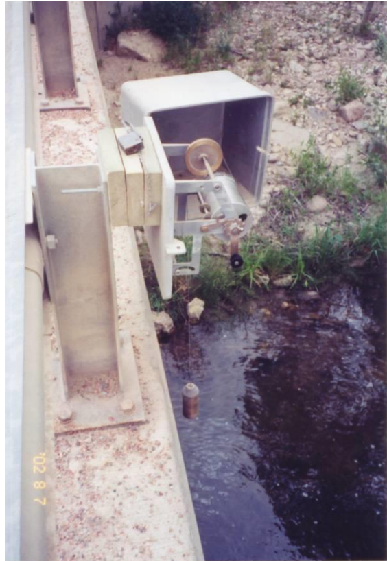
Figure 6-9. Right photograph. Photograph of the USGS wire-weighted gauge used at Big Goose Creek site BG14. Site BG14 was located south of Beckton at USGS Station No. 06302200.
