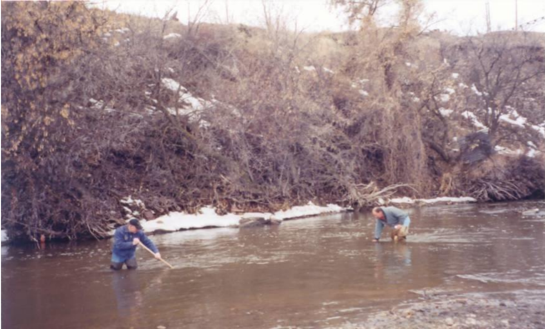
Figure 6-4. Collecting fecal coliform and turbidity samples while disturbing bed sediment with a rake.
