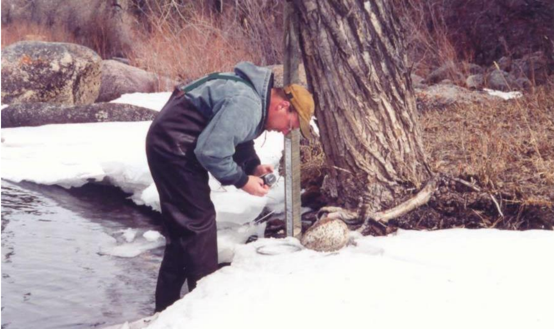
Figure 6-6. Securing a continuous temperature logger casing to a staff guage with stainless steel cable. Station shown is Big Goose Creek site BG18.
