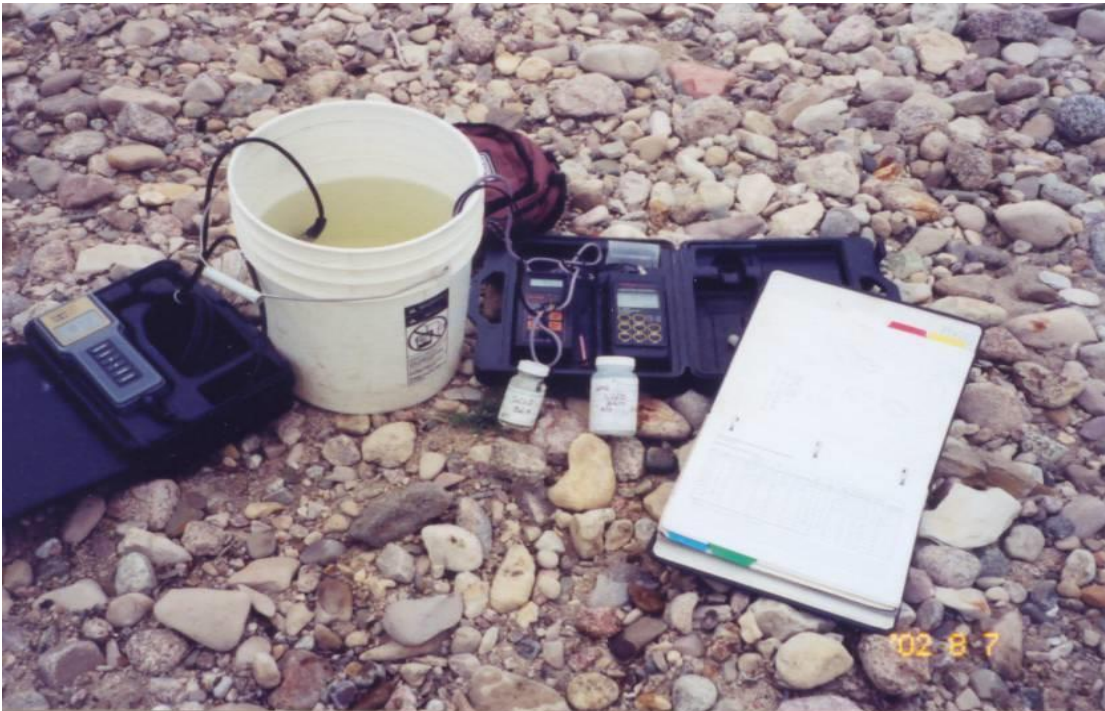
Figure 6-3. Field analysis of pH, conductivity, dissolved oxygen, and temperature. Fecal coliform and turbidity samples are shown near center of picture.
