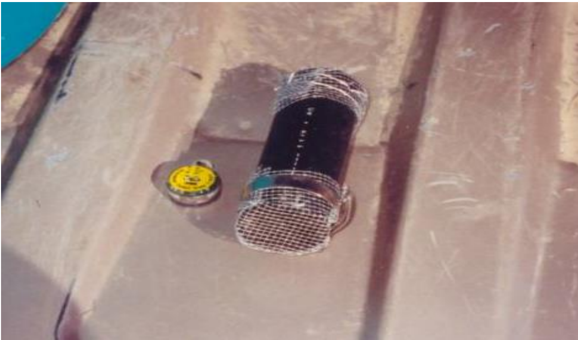
Figure 6-5. Continuous temperature data loggers (left) were secured in plastic pipe designed to allow passage of stream water. The plastic pipe was anchored to a staff gauge with cable.
